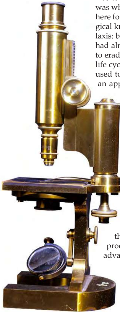
Enrico Verson's microscope, manufactured by Hartnack et Cie of Place Dauphine (Paris). This has two eyepiece lenses and two objective lenses, whose combination provides four different degrees of magnification. Created for a large laboratory, this piece of equipment reflects a period when huge advances were being made in microscope technology. The stand is 26 cm high, the eyepiece tube 18.5 cm long and has an external diameter of 2.5 cm. The two eyepiece (on top) lenses and the two objectives were produced by the Viennese lens manufacturers Reichert.
